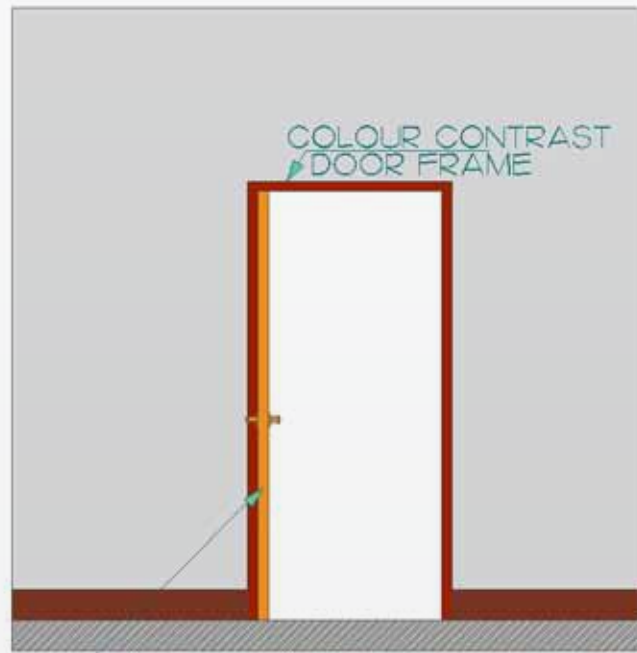
COLOUR CONTRAST DOOR EDGE WHERE DOOR NOT EQUIPPED WITH CLOSER.
