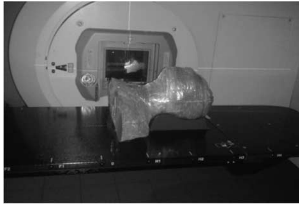
Figure 4. Anatomical Perspex head and neck phantom during 3D-CRT treatment.
