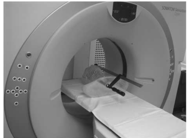
Figure 3. Anatomical Perspex head and neck phantom during CT scan.
